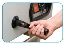
Hand Crank Back Gauge Adjustment Used in conjunction with the LED readout to provide fine control for precision cutting
